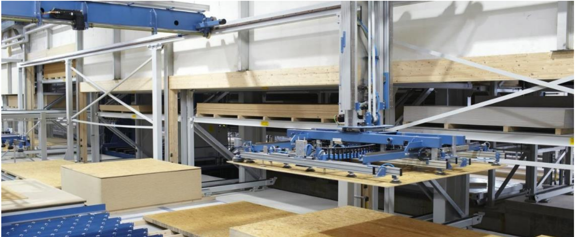
4-axes handling system for plates up to 6 m in length on the set-up station of the ECO 3533 B-Sprint at Renggli
