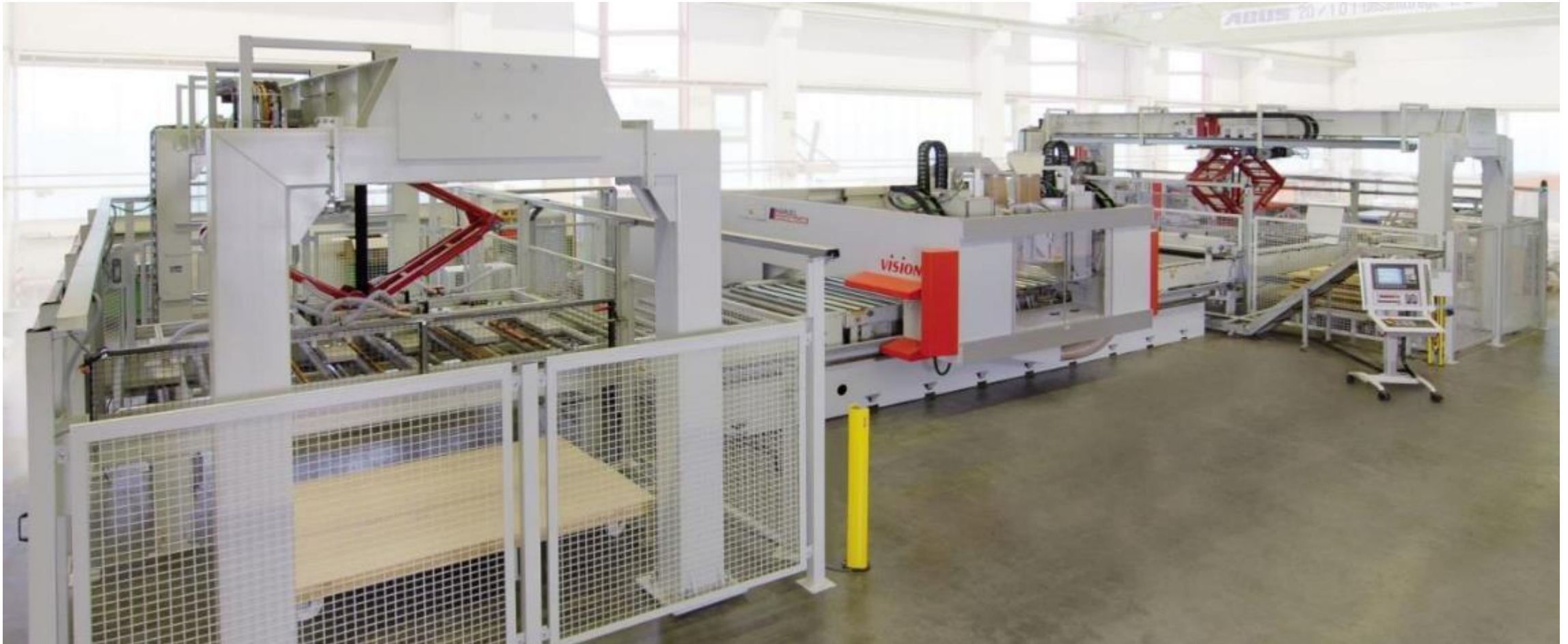
High-tech machining center for efficient door production from batch size 1 to series production
