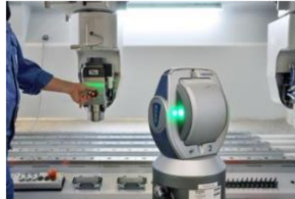
Laser measuring / setting of the machine
