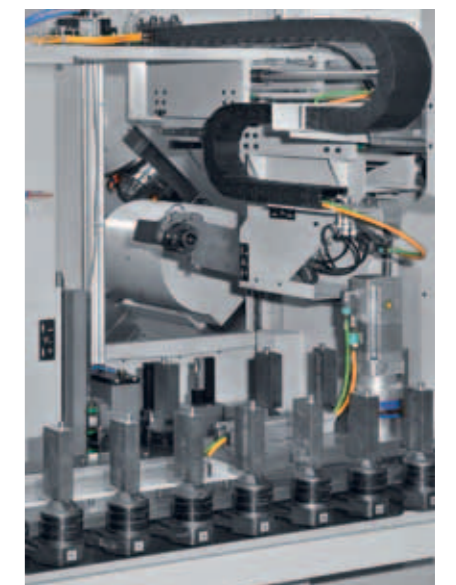
Linear handling by chain magazine
